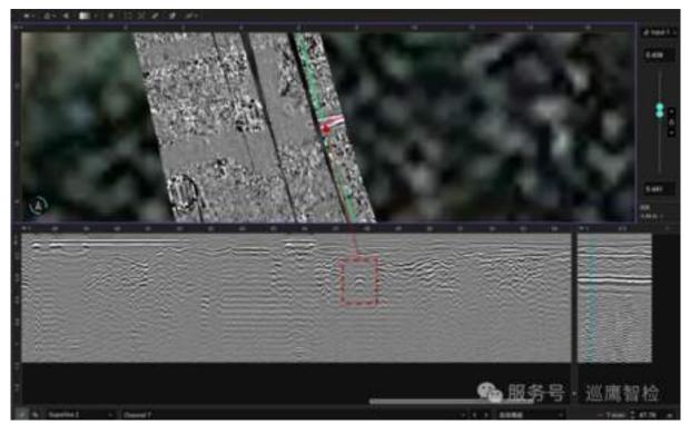
In terms of underground pipeline detection, radar B scan and depth slice showed that there was a reflection signal from a metal pipe at a depth of about 40 cm.
