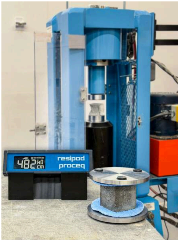
Laboratory setup of Proceq Resipod during bulk resistivity measurement of mortar cubes.
