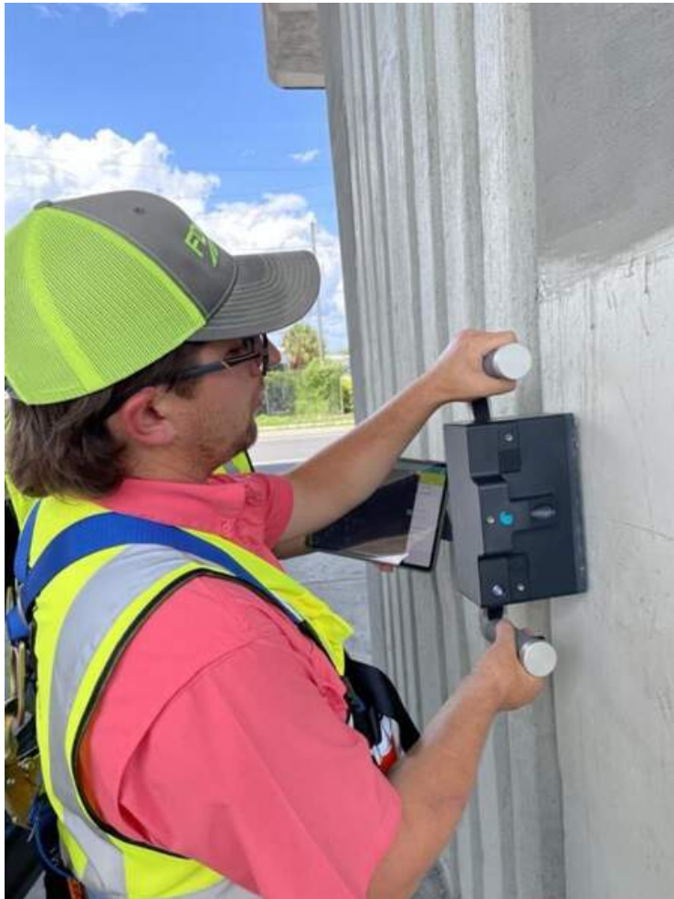
The Pundit PD8050 ultrasonic pulse echo system
