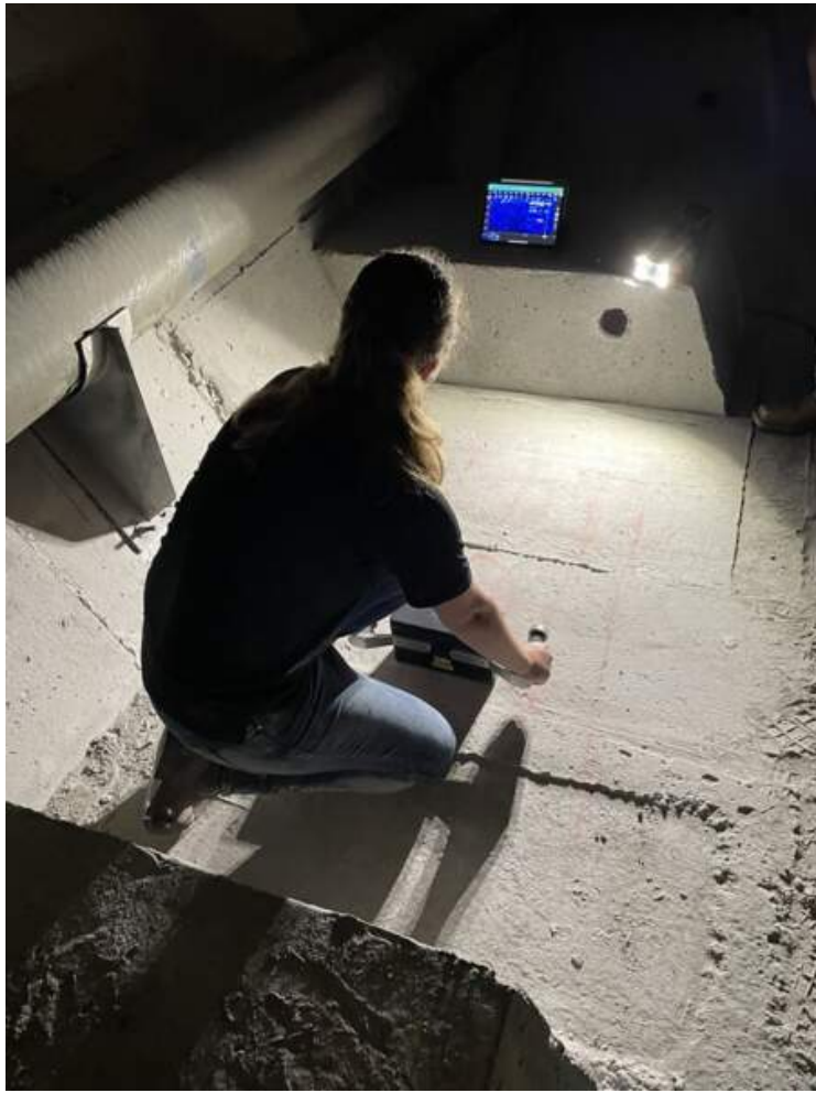
The Pundit PD8050 ultrasonic pulse echo system
