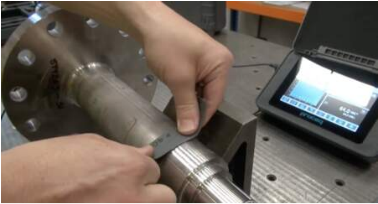
Fig. 5 — preparing the surface with sandpaper
