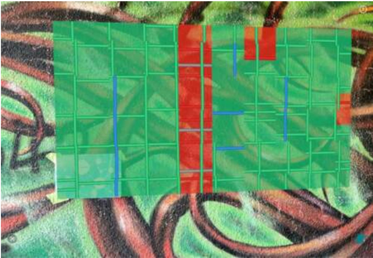
Profometer PM8000 covermeter data viewed with AR projection
