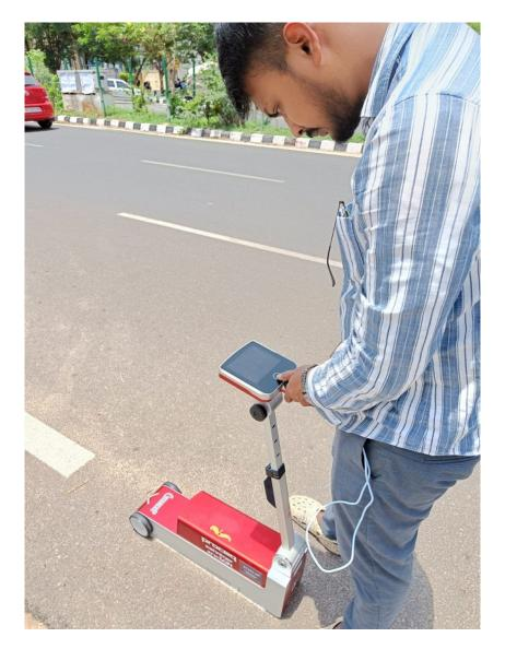
Enabled with 5.7" high-resolution color touchscreen, the retroreflectometer offers excellent visibility under all light conditions. The retroreflectometer logs all measurements with precise geolocation & provides comprehensive reports quickly with the help of user-friendly reporting software at ease.
