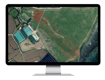
For deeper analysis, the team used <u>GPR Slice</u> post-processing software. In this image, you can see the white lines which represent the distribution of the underground lava cave by 3D scans.
