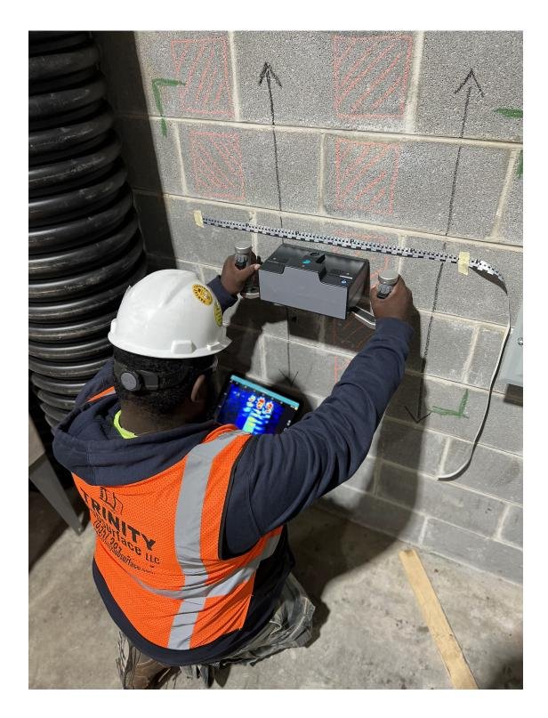
For large areas of different shapes, the team make good use of the Proceq GS8000 Pro's 'free path' feature which allows them to scan the subsurface as they walk freely, unconstrained by a grid.
