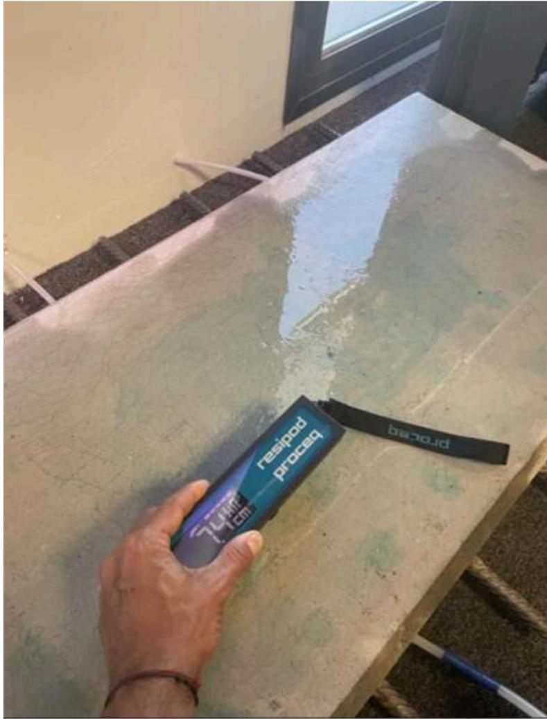
Concrete resistivity results using Resipod
