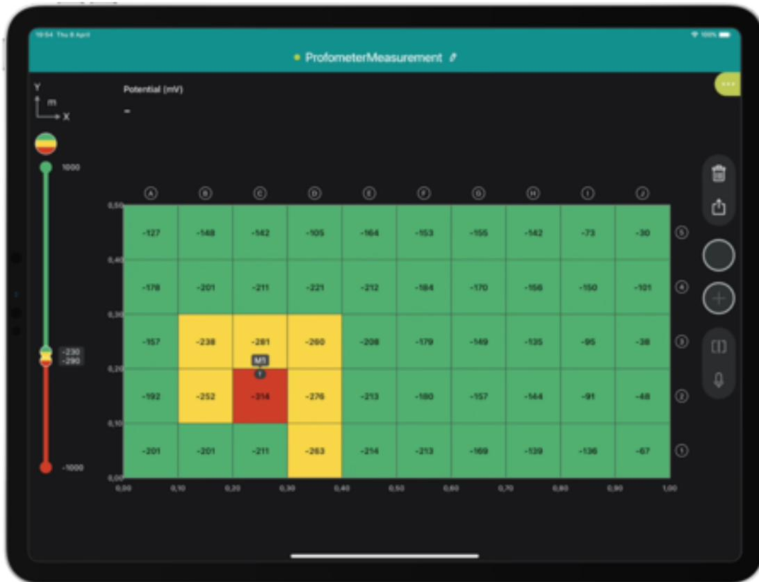
Corrosion likelihood using Profometer PM8500 Corrosion
