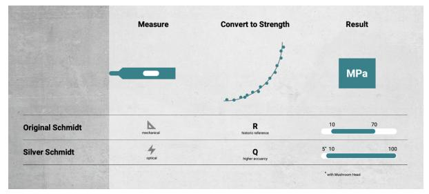
Yes, there are - and this is where the Schmidt Rebound Hammers for the estimation of concrete strength and uniformity come into play. We invented the Schmidt principle over 60 years ago and the method is completely non-destructive.
