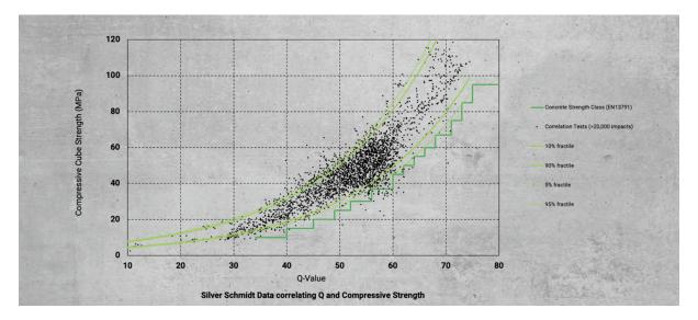
As with obtaining the result from crush tests, the rebound method is also statistical. When used correctly, it gives you more reliable, holistic, and much more cost-effective concrete strength estimation when combined with a few crush tests.
